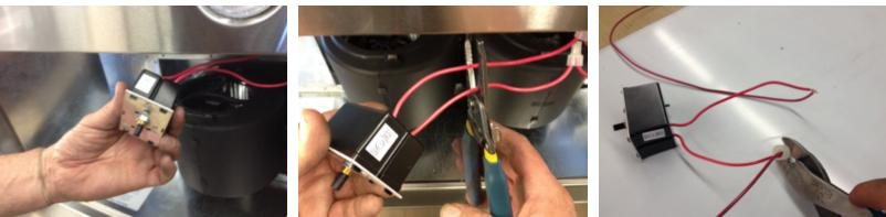
Step 4 Reach behind the panel and pull out the blower switch.
