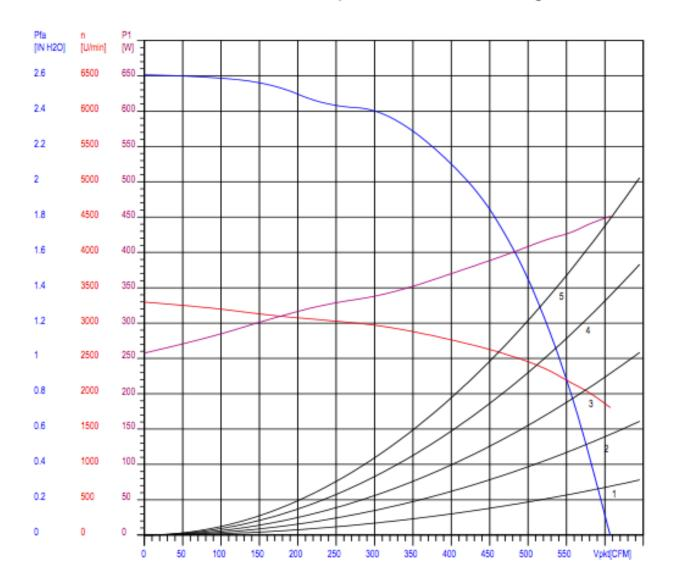
Conclusion: As seen in the above graph, even when long ductwork is used, minimal loss in air flow occurs due to the high back pressure capabilities of the blower.
